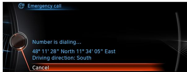
Automatic activation as soon as crash sensors or airbags are triggered.
