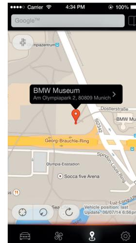
Search for POIs in the third menu item on the lower status toolbar, including the option of sending addresses to yourself in the vehicle. The addresses can be accessed in the vehicle under 'Messages' in the ConnectedDrive menu.
